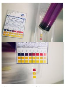
Expel the contents of the syringe to cover the test pads on the pH test strip.
