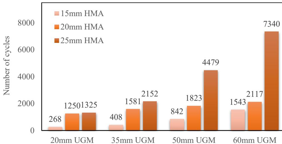
**Figure 5:** Cycle number to initiate cracking in wheel tracking specimens
