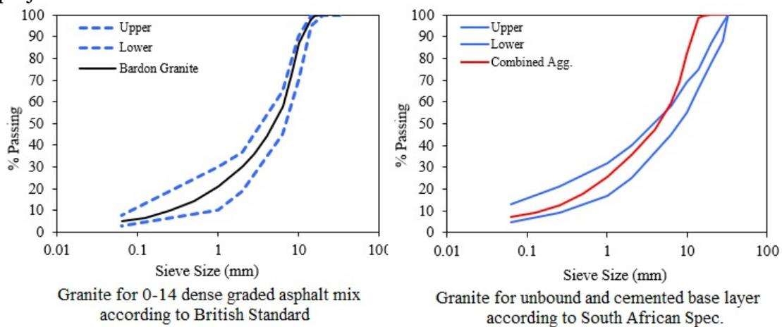
**Figure 3: Aggregate gradations selected for the study**
