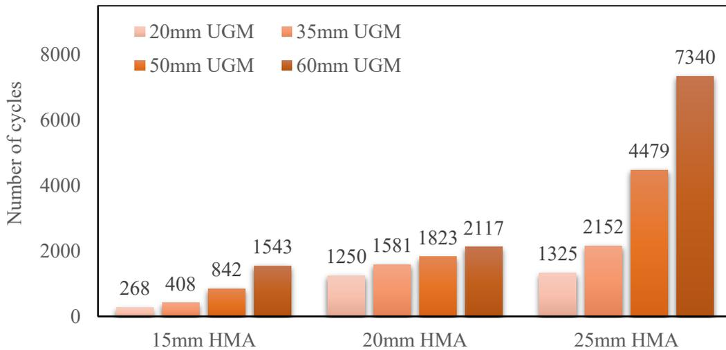
**Figure 6:** Effect of HMA thickness on cracking with varying UGM thicknesses
