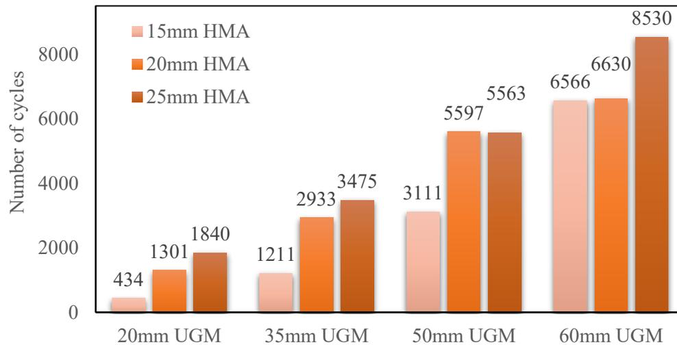
**Figure 7: Cycles to failure on visual inspection**
