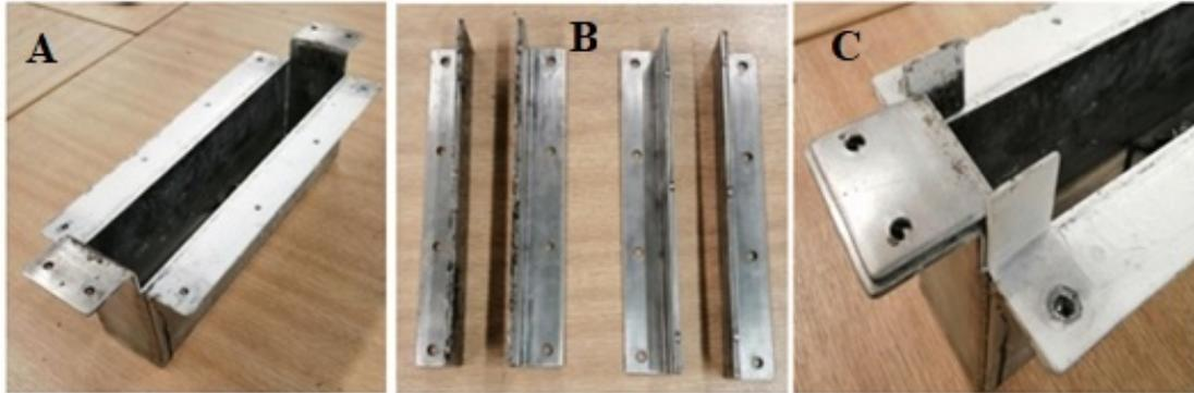
**Figure 4:** New assembled mould and parts
