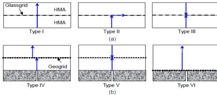
**Figure 2:** Reflective cracking paths observed in: (a) HMA/HMA structure with a glass-grid interlayer (Jayawickrama et al., 1987) and (b) HMA/PCC structure with a geo-grid interlayer (Kuo and Hsu, 2003)
