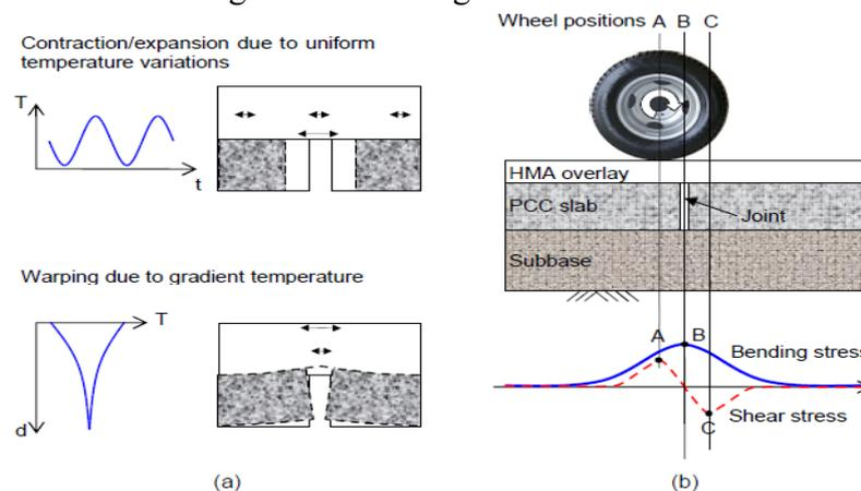
**Figure 1:** Schematic of reflective cracking mechanisms: (a) temperature variation and (b) traffic loading (after Baek, 2010 thesis)
