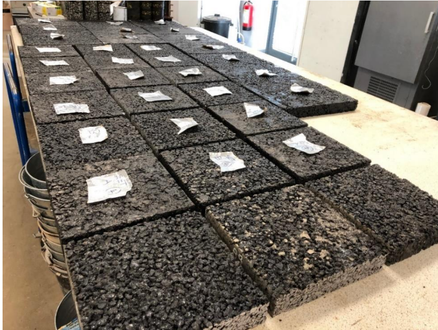
Figure 4. Overview of asphalt samples cut to 260 mm x 260 mm as per DSD testing requirements
