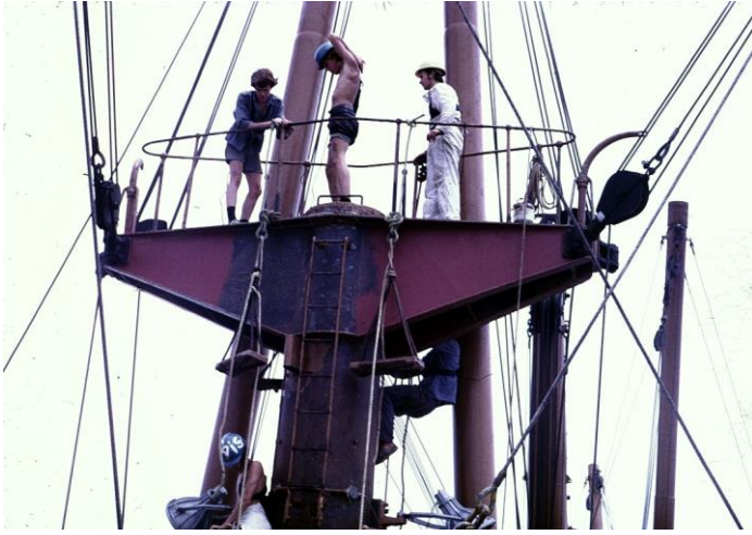
The Training Officer supervising the cleaning and re-painting of the foremast and derricks. Note the jumbo derrick that was forward of this mast.
